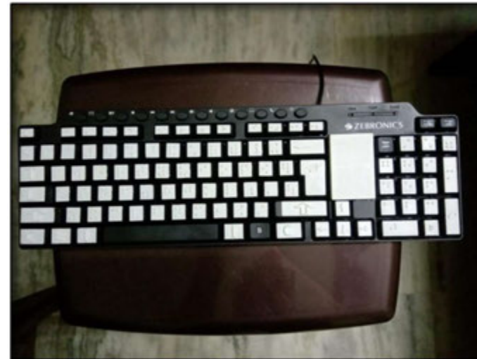
3D printed computer keys and Odia language letter scripts for Blind persons
